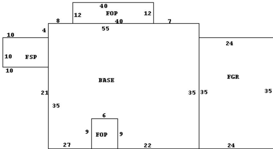
It is critical to the proper coding of structures to supply adequate measurements of the perimeter and auxiliary areas in order to determine the correct location of the auxiliary areas with respect to the base.
