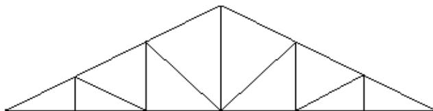
**WOOD TRUSS** - This is made up of various size lumber or timber such as beams, bars, and ties, usually arranged in triangular units to form a rigid framework and may be flat, shed or pitched. Spans are limited due to the strength of the material. This is to be used in place of the flat or shed on commercial buildings with limited spans.
